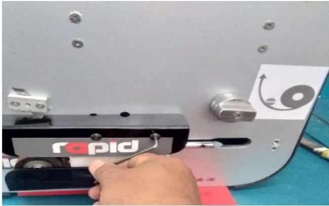
Using Allen Key, unscrew the bolts of the safety cover.
