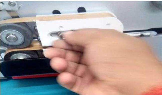
Unscrew and loosen the Bolt of the White Bracket for sliding movement of bracket for easy removal of the belt.
