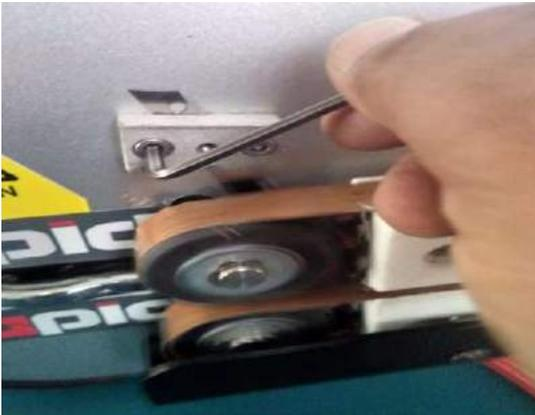
Using Allen Key, unscrew the Left Screw from the Blade Holder
