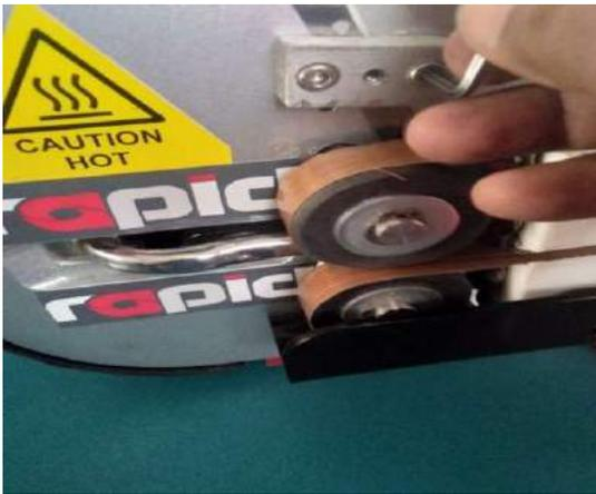
Using Allen Key, unscrew the Left Screw from the Blade Holder
