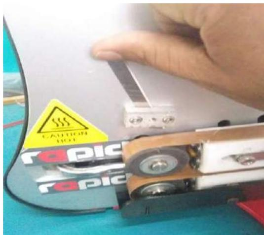
Remove the Blade from the Holder and change the blade and using allen key tighten both the Screws.
